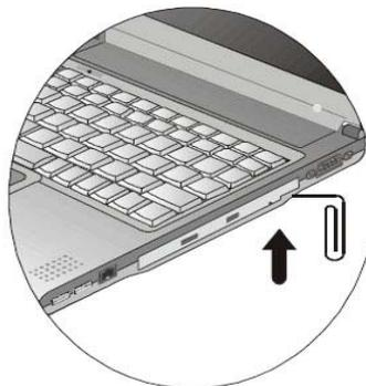
The CD disk tray should eject immediately. This procedure can also be used to remove a CD from the drive when the notebook is powered off.
