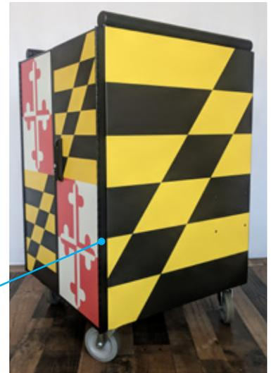
Note that door hinges on left and right side need to be exposed, so the side skins are not mounted flush against the door skins
